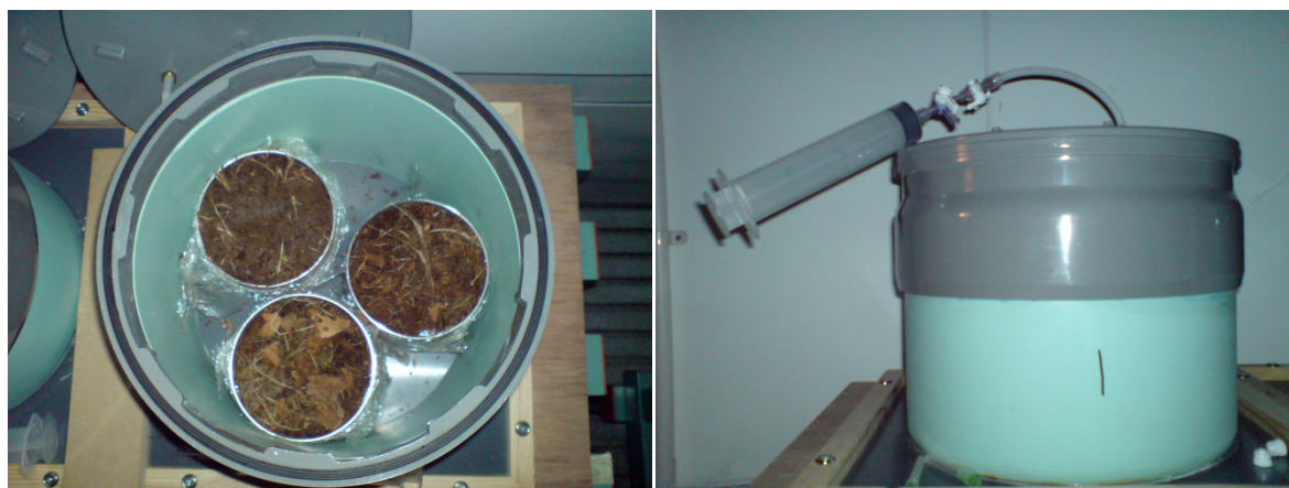
Figure 2.3: Closed-chamber set-up for the measurement of net CH 4 fluxes.
